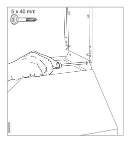
■ Secure the canopy with 5 x 40 mm screws into each drilled hole.
